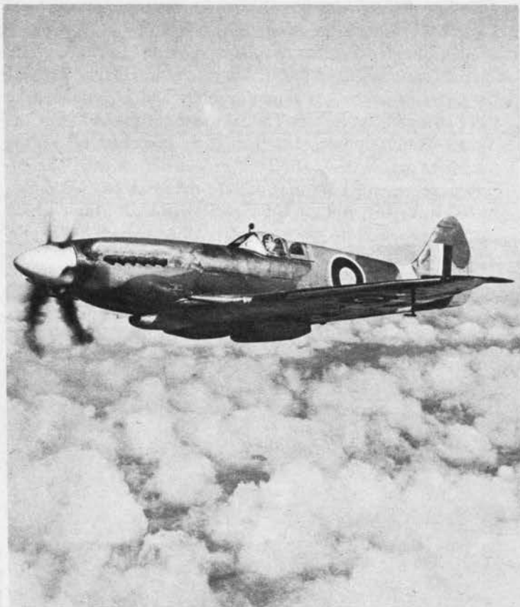
Huge spinner houses control mechanism for the new five-bladed propeller. The nose, tail and wing outlines retain familiar smooth curves.
